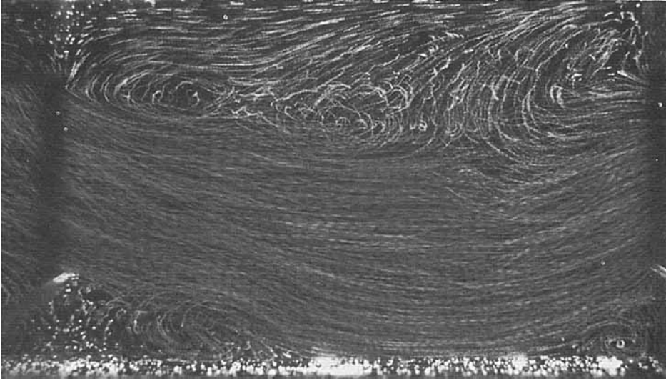
FIGURE 10. Experimental streakline photograph for Re = 359 . Exposure time = \frac{1}{8} s.
